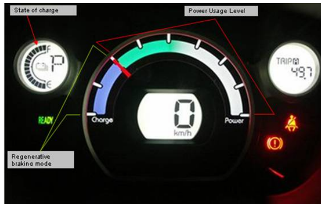
Figure 3.65: i-MiEV instrument cluster
