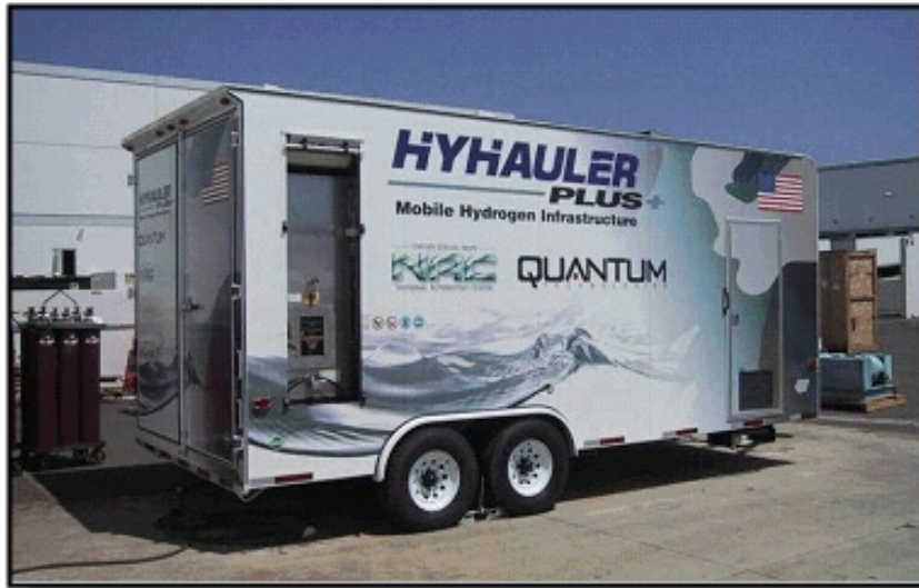
Figure 9.31: Mobile On-Site hydrogen production and dispensing unit
