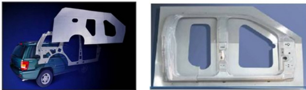
Figure 10.2: Laser welded blank to final stamping example
