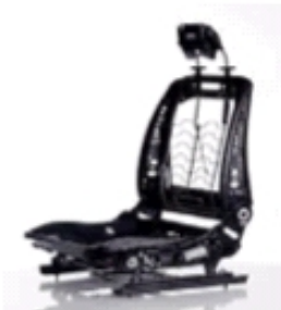
Figure 11.31: The front seat frame structure consists of 65 to 70% of total seat mass
